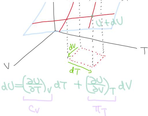
Define internal pressure to be  $TT = \left(\frac{\partial U}{\partial V}\right)_{T}$ ; same units as pressure dU = CVdT + TT - dV
