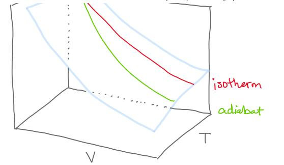
in an adiabatic process, the pressure drops more quickly compared to an isothermal process with the same initial conditions.
