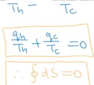
Efficiency  $\eta$   $\eta = \frac{\text{work performed}}{\text{heat absorbed}} = \frac{|\omega|}{|q_h|}$   $\eta = \frac{|q_h| - |q_c|}{|q_h|} = 1 - \frac{|q_c|}{|q_h|}$   $\eta = 1 - \frac{T_c}{T_h}$   $1 - \frac{15}{20} = 25\%$
