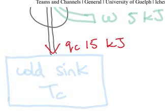
A certain power station operates with superheated steam at 573K and discharges the waste heat into the environment at 293 K. What is the theoretical efficiency?  $\eta = 1 - \frac{T_c}{T_h} = 1 - \frac{293}{573} \approx 48.9\%$
