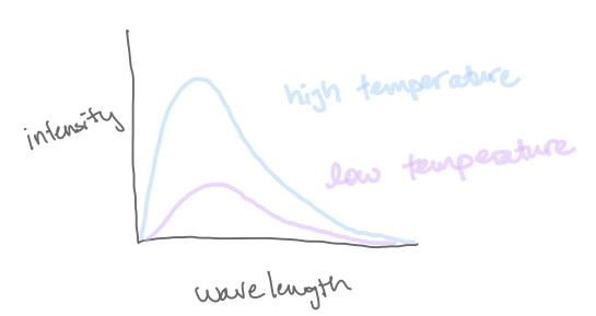
an experimental Construction -> measure radiation that is emitted Postulate: a blackbody is as good at absorption as emission suppose dackbooks this darks it emits but, this would violate the second law of thermodynamics! Many entities are approximate blackbodies, including humans!
